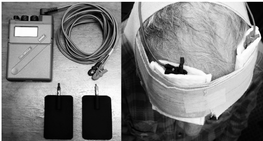
Figure 3. The tDCS was delivered using the Chattanooga Ionto™ Dual Channel Iontophoresis System and 4 x 6 cm conductive rubber electrodes as shown in the left image. The right image shows the electrodes placed in saline-soaked sponges and secured on participants' heads with bandages.
