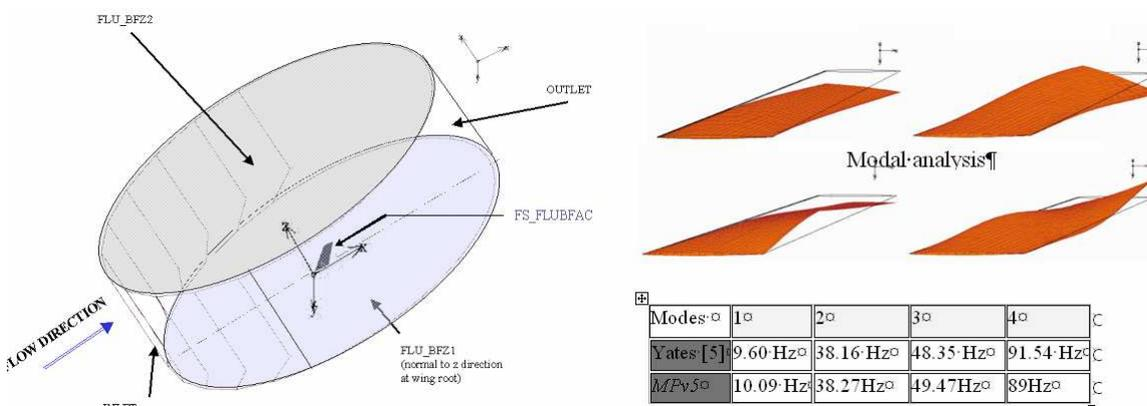
FIG. 1 – Computational domain and structural mode computation of the clamped Mahogany wood wing of AGARD445.6 Wing.
