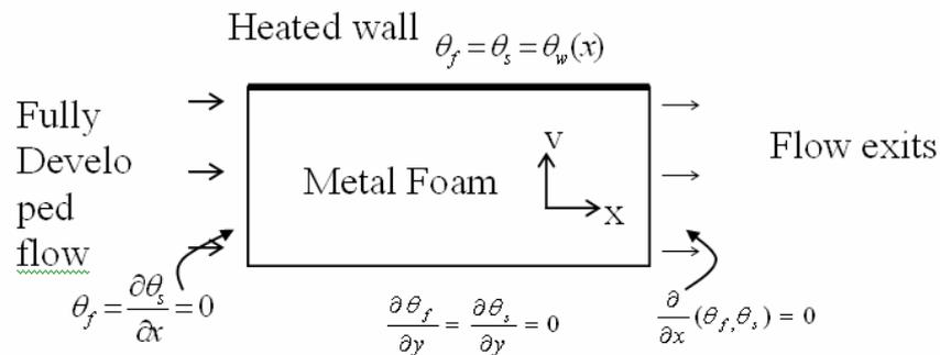
FIG. 5 – Fluid Schematic for the flow through and around a porous structure: Geometry and FSI mesh
