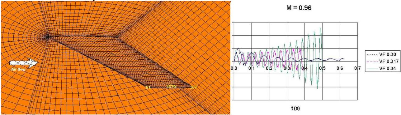
FIG. 2 – Trace point of the structure at tip of the wing, and displacement record for different  $V_f$  values
