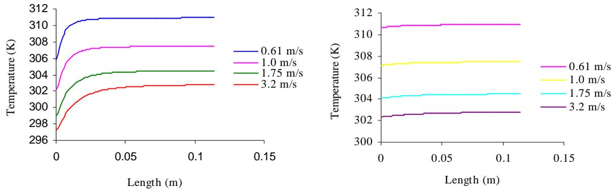
FIG. 7 – Longitudinal variation of temperature in the fluid (left) and solid (right)
