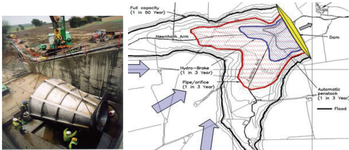
(b) Flooding areas for different flow controls and storm events (adapted from Boakes et al. , 2004)
