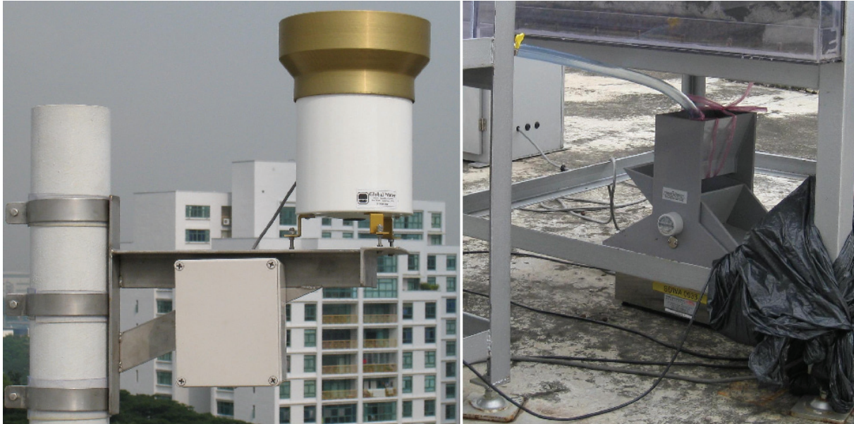
Figure 3 Experimental setup of the rain gauge (left) and flow gauge on weighing scale (right).
