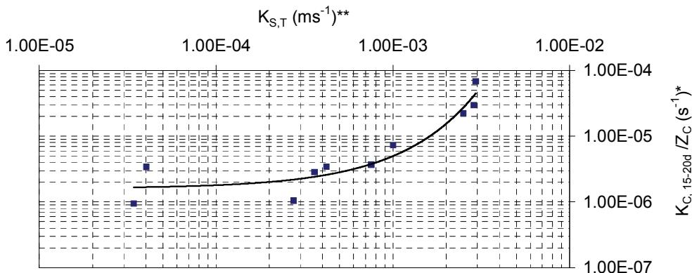
\* mean leakage factor after 15-20 d clogging; \*\* hydraulic conductivity of the backfill potential height: 0.1-0.2 m; maximum particle size of the waste water: 0,5 mm
