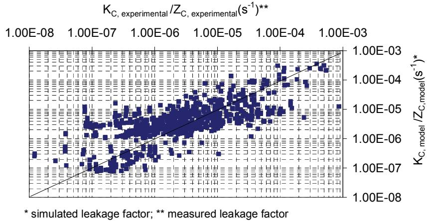
Figure 2: Measured and simulated leakage factors
