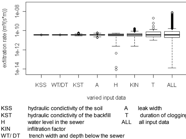
Figure 5: Exfiltration rates under dry-weather conditions as a consequence of variation of input data
