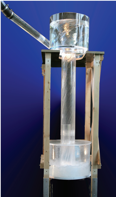
Fig. 3. The 1:10 scale model test. The second feed pipe opens out into the vortex chamber from the rear, it is not visible from this view.
