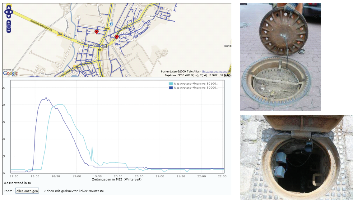
Fig.5: HydroWebView showing the available runoff data in the catchment of Prenzlau
