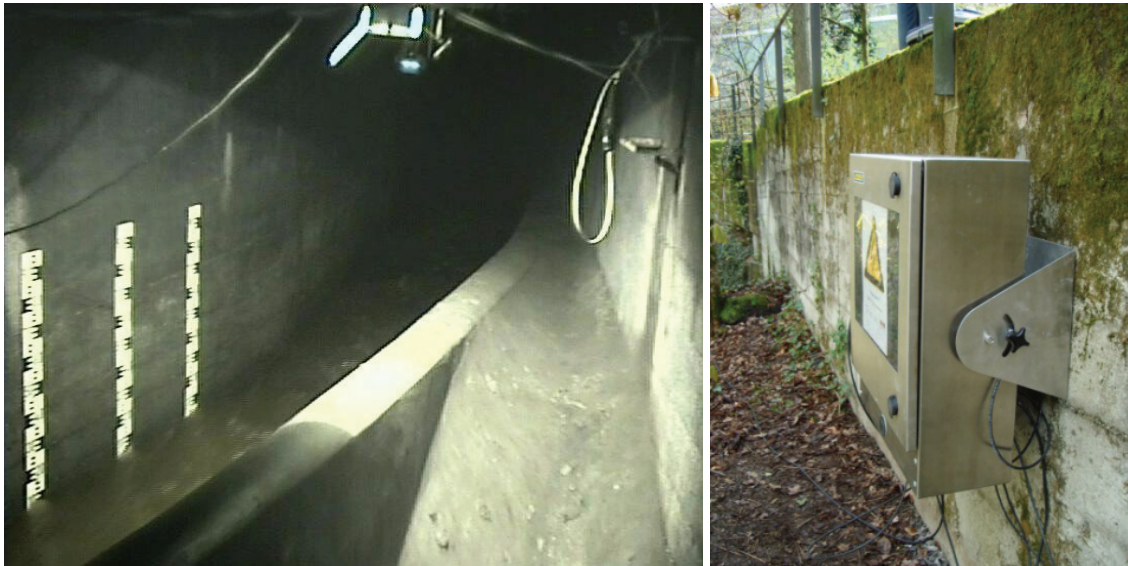
Figure 1. Left: View of a combined sewer overflow with infrared illumination system. Rulers are strongly fixed on the wall to validate water level measurements and for camera calibration. In case of high rain events, some waste can hang on the ruler, and cleaning is required. Using images, we can directly see if a such operation is needed (by our experience, we have to do that only one time a month). Right: Example of installation for the acquisition system that remains outside of the sewer system to facilitate the access and to avoid problems in case of flooding events
