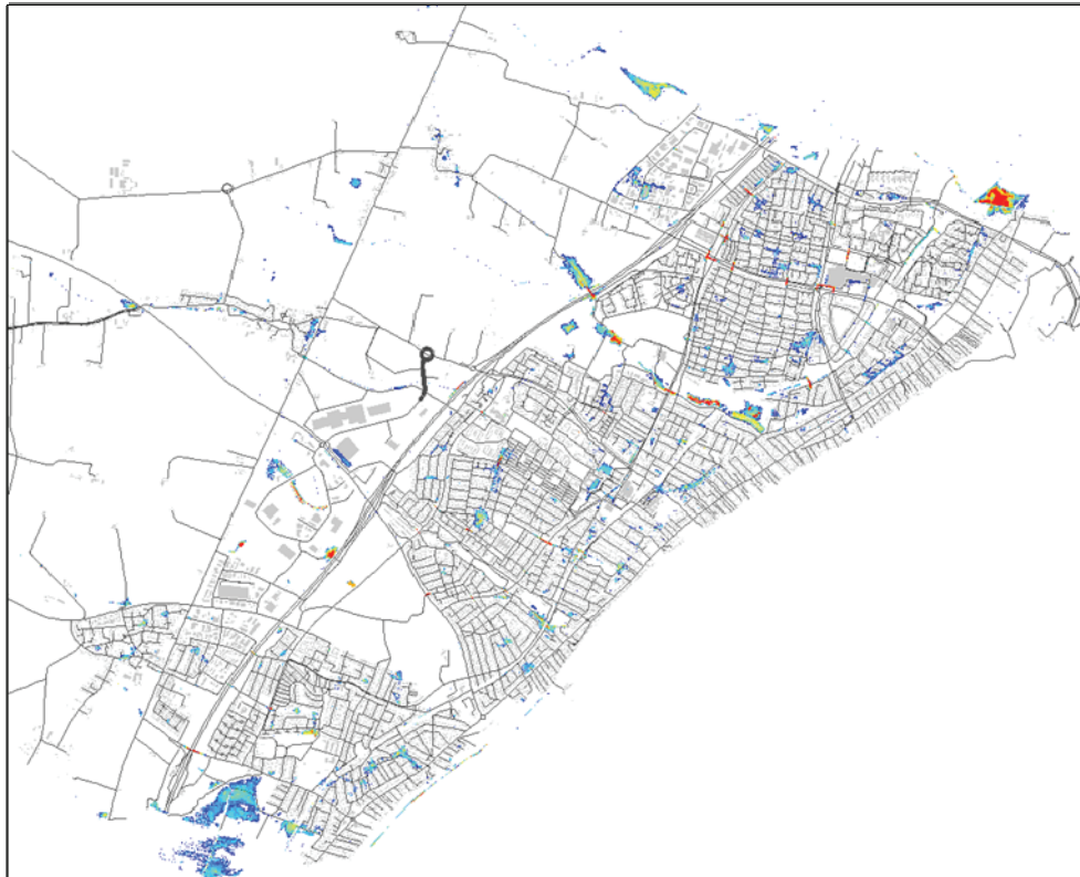
Figure 9. Example of a simulation of flooded areas for a specific return period displayed in the GIS environment.
