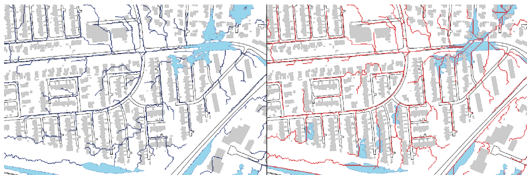
Figure 1. Difference in flow paths and calculated ponding areas when using a DTM (left) or DSM (right) as input.
