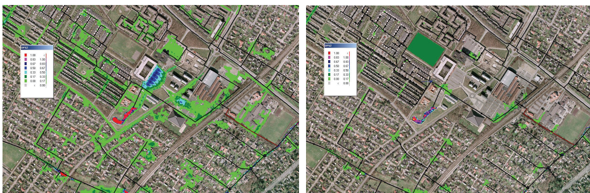
Figure 7: Extreme rainfall. Left: without activating an emergency plan. Right: Activating an emergency plan.
