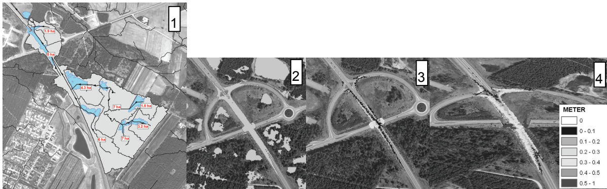
Figure 8. Risk area identified (1). Depression using level 1 (2). Calculated maximum water depth for T = 100 years (3). T=500 years (CF=1.4) (4).
