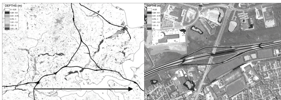
Figure 5. Examples of blue spots, which has information about area, volume and depth.
