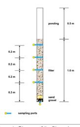
Figure 1. Diagram of the filter columns
