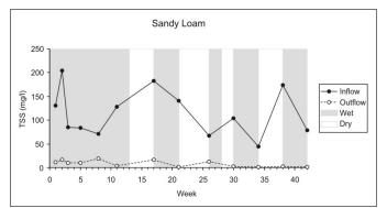
Figure 2. Mean inflow and outflow sediment concentrations from the sandy loam filter columns
