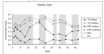
Figure 3. Mean inflow and outflow concentrations of phosphorus from the sandy loam filter columns
