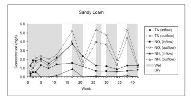
Figure 4. Mean inflow and outflow concentrations of nitrogen from the sandy loam filter columns
