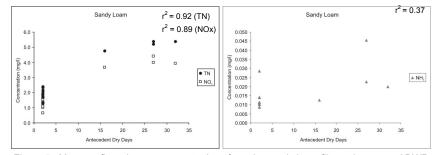
Figure 5. Mean outflow nitrogen concentrations from the sandy loam filter columns vs. ADWP
