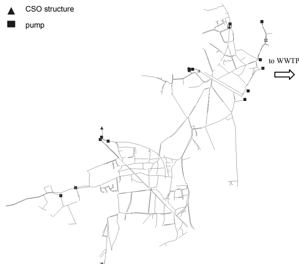
Figure 1: Overview on the sewer network of Herent
