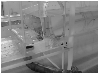
Fig.5. Laboratory investigations on Septurn diverter: a) model during detention phase b) results comparison between measured and calculated values of h_R for varying mass of counterweight.
