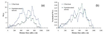
Figure 1. Width functions for pre- and post-development conditions: (a) Comparison of the width functions, (b) Comparison of the normalized width functions.
