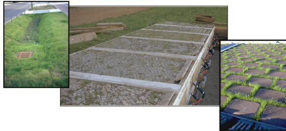
Figure 4 Research of the pavement area for active infiltration (Schmidt, 2004)
