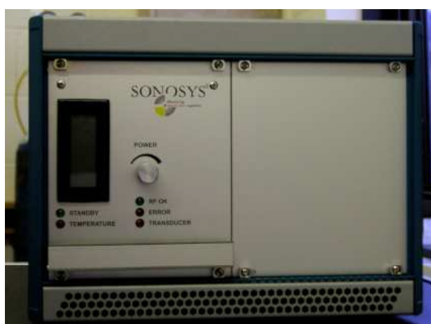
Fig. 1 Megasonic generator. 500 W Electrical power at 1MHz
