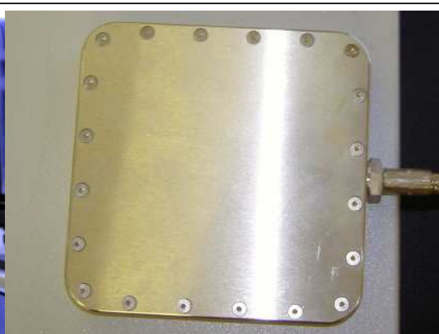
Fig. 2 Megasonic transducer of 4 by 4 inch active area
