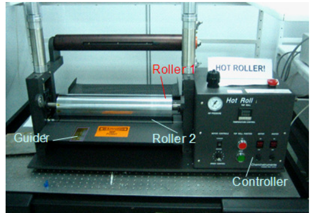
Fig. 1. The micro roller embosser used in this study. Roller 1 was a driving roller with an embedded heater inside; and roller 2 is a supporting roller made of hardened rubber.
