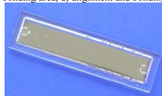
Figure 5. Photo of the microfluidic chip for RBCs trapping
