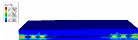
(b) Stress distribution at device wafer thickness 100um case
