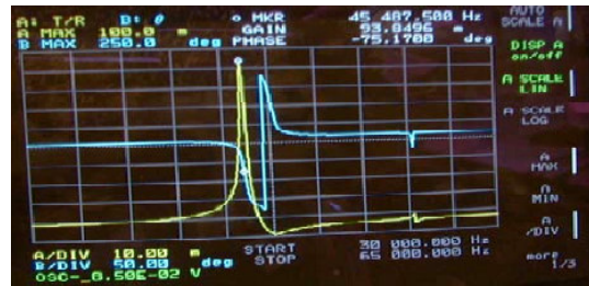
Fig. 6: Gain (0.093) and phase of a beam micro transformer using an uniform AlN film on the primary (input) and secondary (output) electrodes
