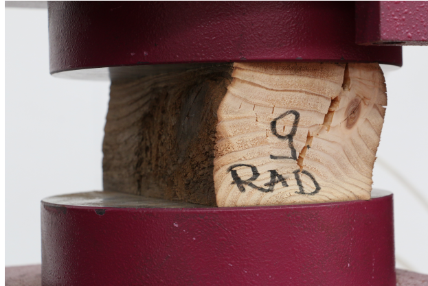
Figure 7: A sample under radial compression.
