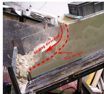
FIG. 6 Slip surface from one side of tank.
