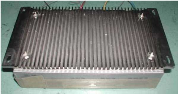
Figure1. Vapor chamber with optimal fin design
