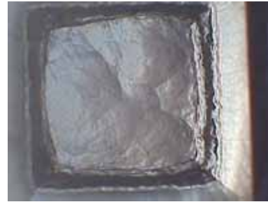
Figure 3. After etching (50% KOH at 95 ^\circ\text{C} for 4 hours) structure for a 1 \times 1 \text{mm}^2 etch window
