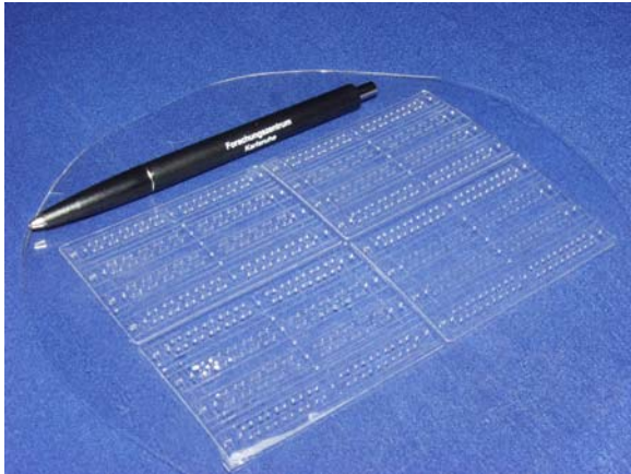
Figure 3: Molded part of the 8-inch microstructured mold.
