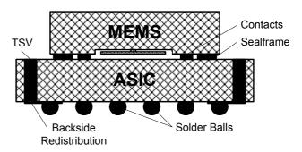
Related technology elements are suitable metallization stacks, passivation technologies and conformal coating in deep etch holes. Effects of process technologies on MEMS functionality and ASIC performance are evaluated by simulation and characterization of a specially designed test vehicle.
