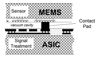
Local mechanical stress from the bonding process acts directly onto the processed structures. Countermeasures against damage and functional deterioration must be developed on design level and in form of technology optimization. A high involvement of CMOS design and integration experts, equipment suppliers and academic partners in the DAVID project shall lead to a set of design rules addressing the potential risks.
