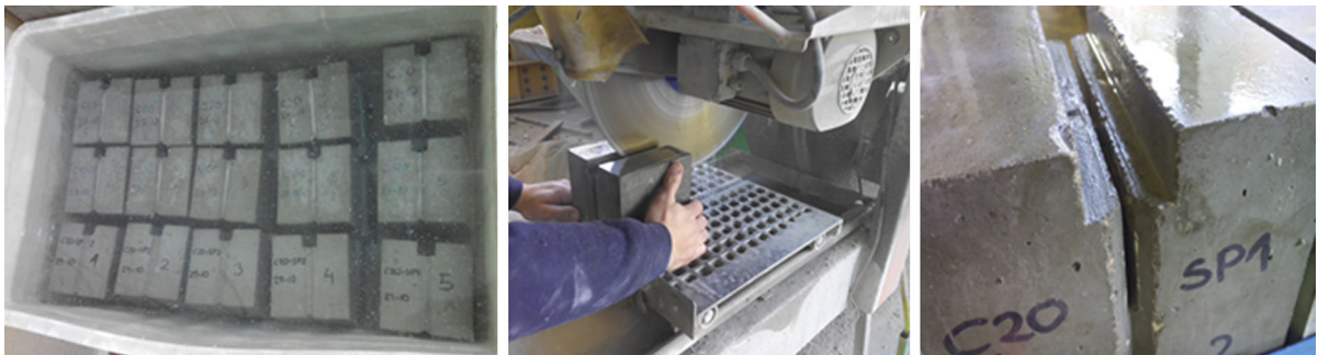
Fig. 3 Specimens curing and notches sawing
