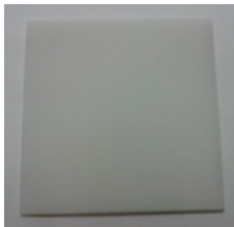
Figure 4. Optical epoxy phantom with TiO 2 embedded nanoparticles.
