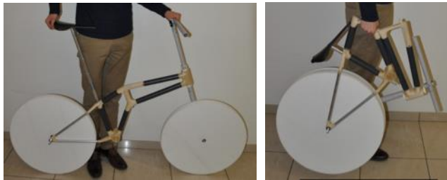
Figure 4. First quick and dirty full-size proof of concept.
