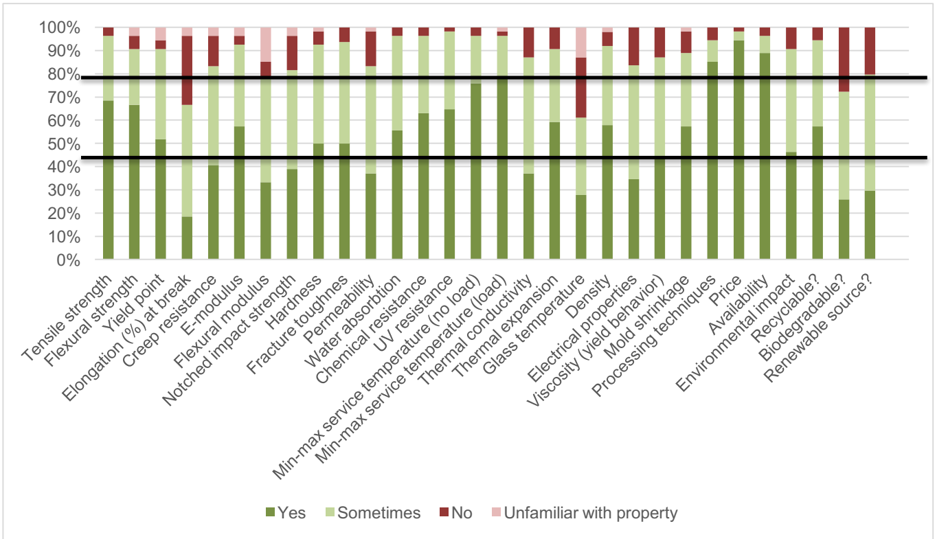
Fig 2. Results of the survey regarding the relevance of the proposed material properties.
