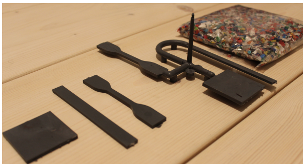
Fig 4. Test bars used for standardised testing, made from recycling flakes.
