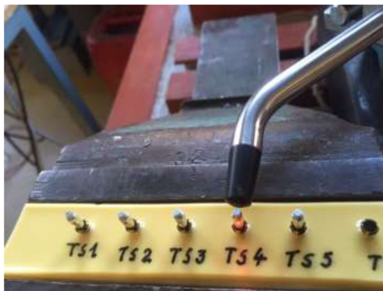
Fig. 2 Clamped Osstell probe orientated towards a Smartpeg mounted on a test implant. Note the red laser beam dot on the flat surface of the Smartpeg hexagon part
