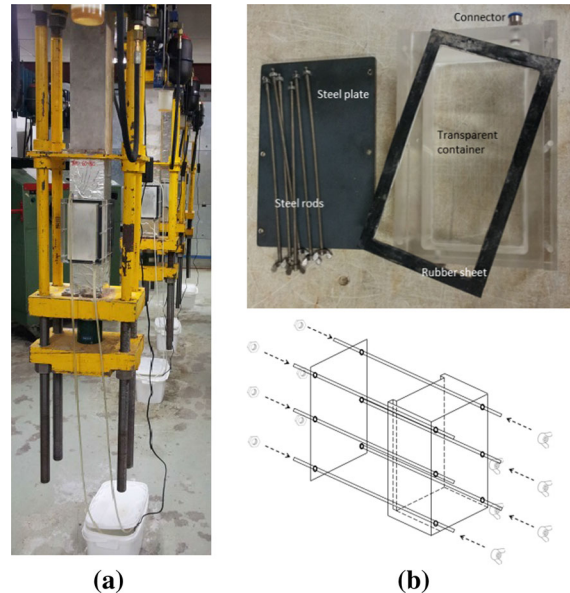
Fig. 2 Details of test equipment: a example of test rig with specimens including attached container for chloride solution, and b container and principle for fixation of container
