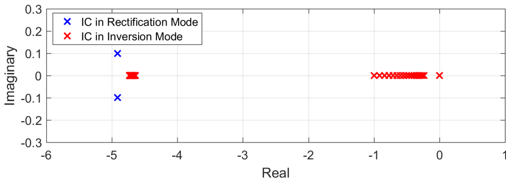
Figure 6-11: Trajectory of the eigenvalues as a function of DC active power droop coefficient based on Current controller.
