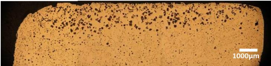
Fig. 6. Upper part of the metallographic section of a sample cooled at 20°C/min.
