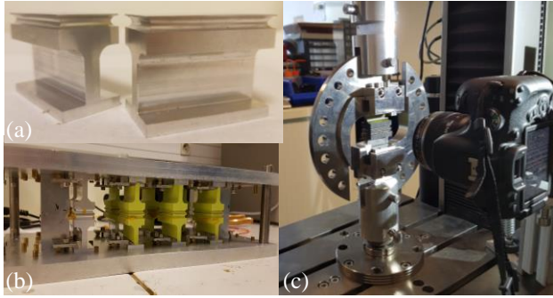
Figure 1. a) ARCAN test specimen; b) Experimental device to mold ARCAN specimens; c) Experimental ARCAN setup
