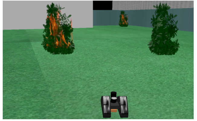
Fig. 2. Simulation of the robot in its environment with MORSE
