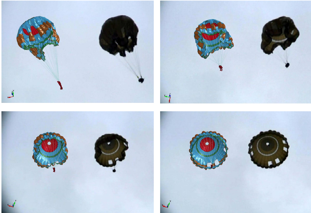
Figure 14. Real and computed profiles compared at different times during the opening.
