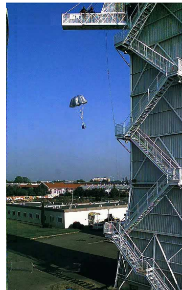
Figure 9. Drop of a small hemispherical parachute.
