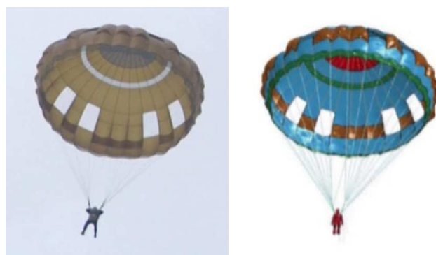
Figure 5. Real and simulated inflated profiles of the EPC.
