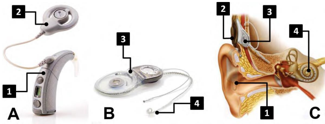
Figure 3 The essential components of a conventional cochlear implant.
