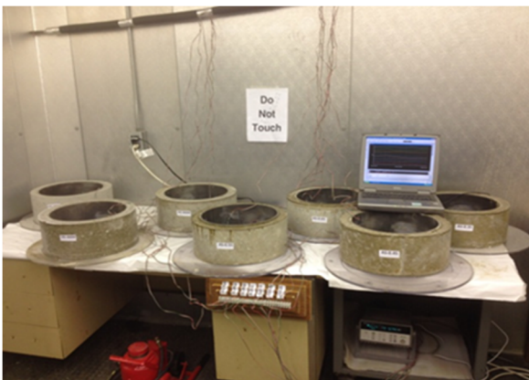
Figure 1. Test setup for strain measurement
