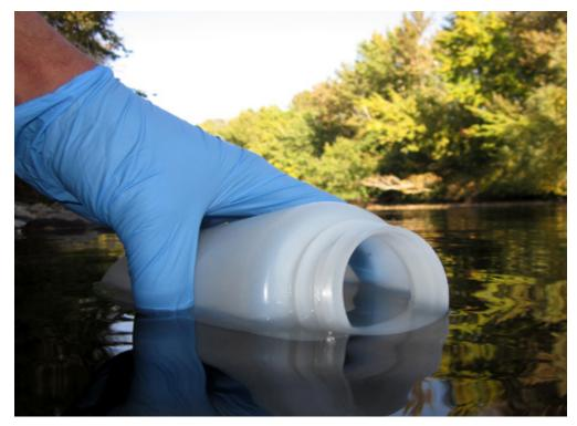
shaking, and then discarding the rinse water away from the location of sample collection. Water samples should be collected by submerging the bottle ½ to 1 foot below the water surface, at a spot several feet away from the edge of the pond, filling the bottle completely, and tightly sealing it with the cap.
