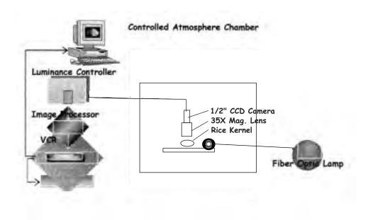
Fig. 1. Schematic of the video microscopy system.
