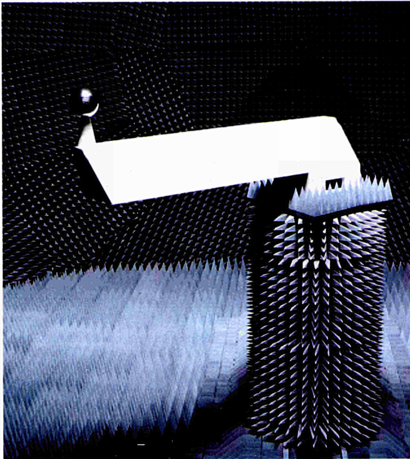
Fig. 6.4. Verification of the "Quiet Zone" of the EMSL using a metallic sphere as a probe mounted on a rotating arm
