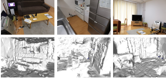
Fig. 5. Examples of input images (top) and reconstructed 3D model (bottom).
