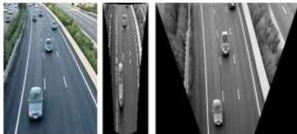
Fig. 4: a) Original image with perspective effect, b) Remapped image that removed perspective with IPM, c) Remapped image that removed perspective with MIPM
