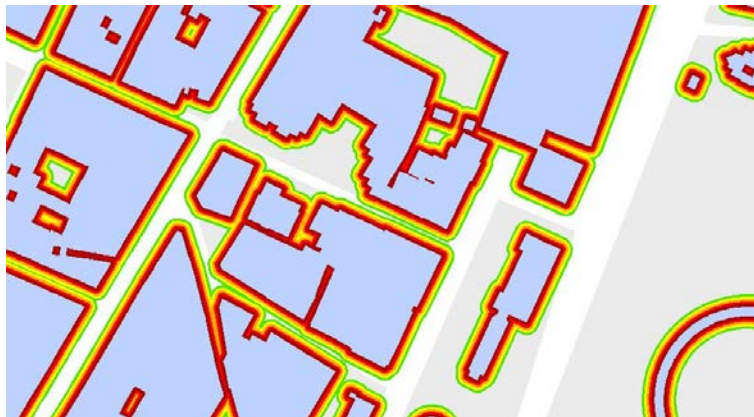
Fig. 7 – Buffers for allocation of debris falling from buildings (blue) to the sidewalks (gray) and roads (white). Red, yellow and green colors denote large, medium and small amount of fallen debris.
