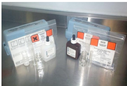
Figura 5.24. Hardness Total Test Kit 5-EP mg/L y Alkalinity Test Kit AL-AP mg/L
