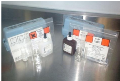
Figura 5.11. Hardness Total Test Kit 5-EP mg/L y Alkalinity Test Kit AL-AP mg/L
