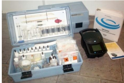
Figura 5.12. Complete Water Quality Laboratory DREL/2400
