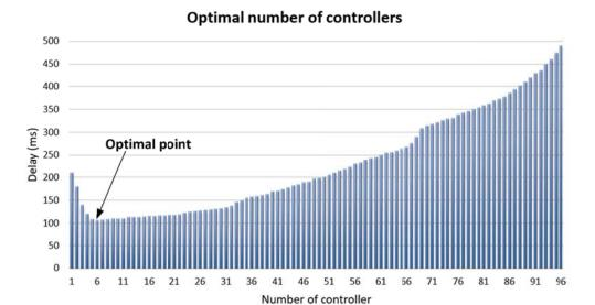
Figure 14: Optimal number of deployed controllers
