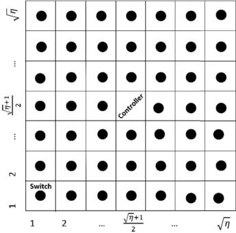
Figure 6 A controller is deployed in the middle of the grid and all  $\eta$  switches are assigned to this controller. Then, the average number of hops 'h' from a switch to controller is  $\sqrt{\eta}/2$  (approximately)
