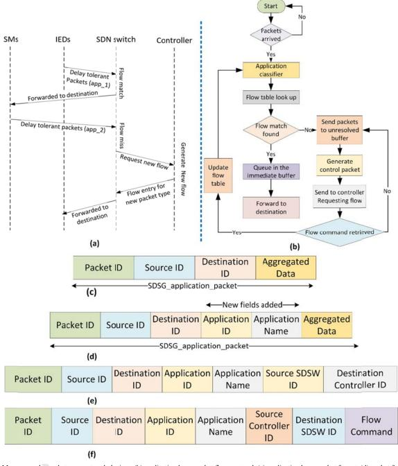
Figure 3: (a) Message exchange between network devices, (b) application layer packet flow protocol, (c) application layer packet format, (d) packet format after application classifiation (e) packet format with flow command request to the controller (f) packet format with flow command form the controller
