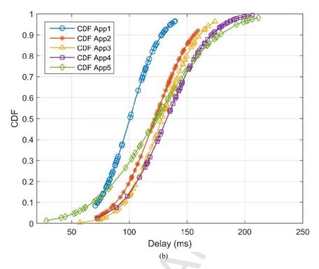
Figure 11: (a) Delay profile of different applications in random scenario (b) Packet delivery time taken by different applications in random scenario
