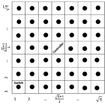
Figure 6: Hop counts in a virtual grid
