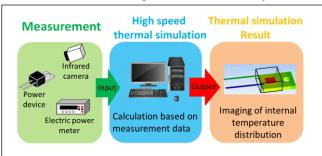
Fig. 1 Principle of temperature distribution imaging by teal-time simulation.
