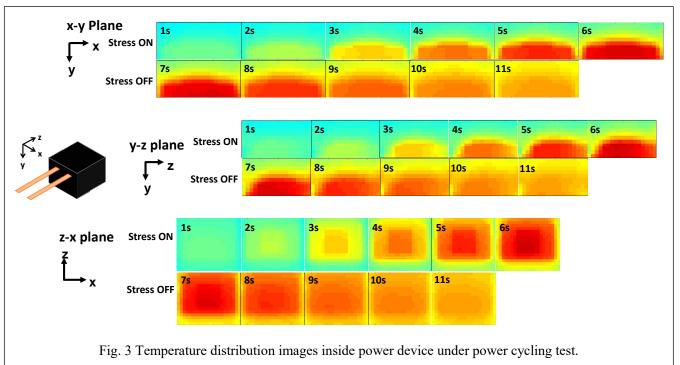
device with 5 s turn-on and 5 s turn-off. Surface temperature ence within 2 °C.
